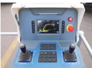
平台控制箱 配备两轴防误操作手柄、背光按键面板、高清显示屏、急停开关等 Platform Control Box Equipped with 2-axis anti-misoperation joystick, backlit key panel, high-definition display, emergency stop switch and other components.
