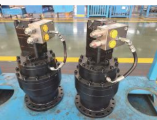
外啮合行星式回转减速机，大扭矩，回转平顺；啮合间隙可调，磨损补偿，经久耐用 External meshing planetary slewing reducer delivers high torque and smooth slewing performance. Its adjustable meshing clearance enables wear compensation for long service life.
