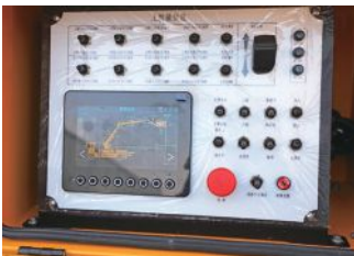
下车电控箱 可操控车辆全部动作，并监测车辆工作状态 Chassis Electrical Control Box Enables full vehicle motion control and real-time monitoring of operating status.
