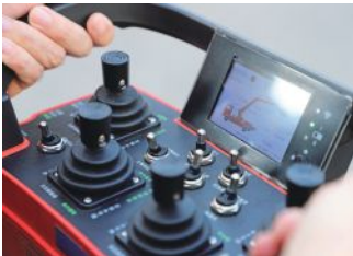
多功能遥控器 远距离操控支腿、臂架、作业平台，操控安全便捷 Multi-Functional Remote Controller Remotely control outriggers, booms and working platform with safe and convenient operation.
