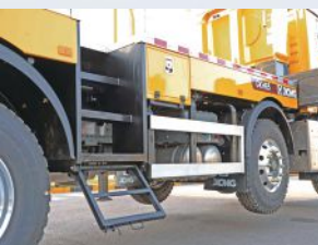
上下车梯（带抽拉梯） Upper & Lower Access Ladder (with Pull-Out Extension Ladder)
